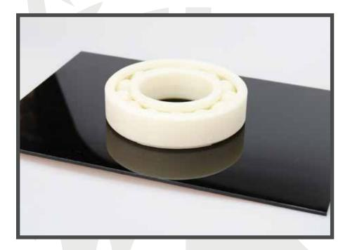
AS PARTS COOL THEY WILL BEGIN TO "POP" OFF OF THE GLASS. DO NOT BE ALARMED, AS THIS IS JUST THE SOUND OF THE PARTS RELEASING THEMSELVES FROM THE WOLFBITE SOLUTION. COLD WATER WILL SPEED UP THE PROCESS, BUT MAKE SURE TO LET THEM COOL IN AMBIENT AIR FOR A FEW MINUTES FIRST.
