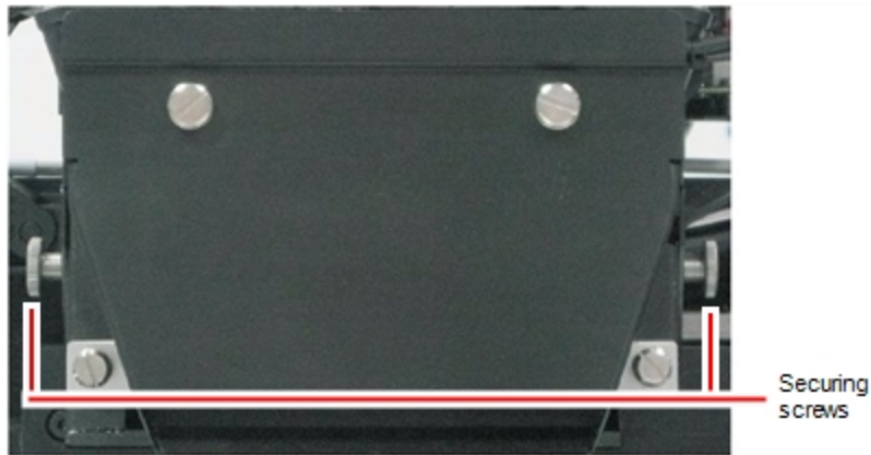
Figure 6-45 UV-lamp-assembly securing screws
