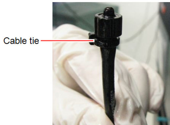
Figure 6-113 Tube with cable tie and fitting
