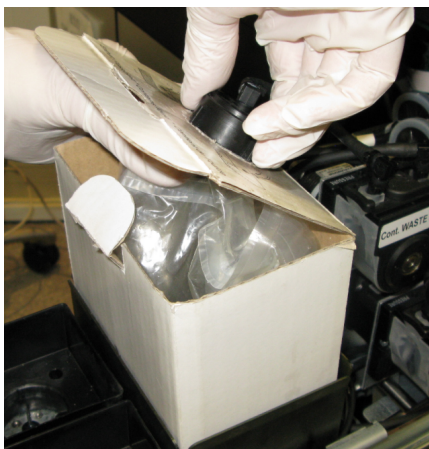
Figure 6-135 Waste container with waste tube attached
