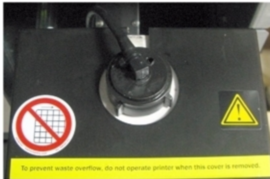
Figure 6-143 Fireproof cover installed over the waste container
