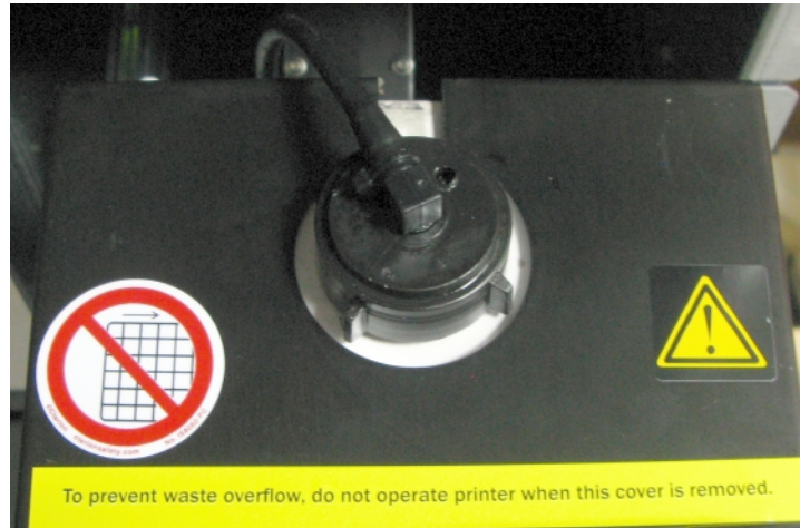
Figure 6-120 Cover installed on the waste container
