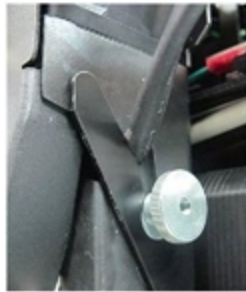
Figure 6-50 UV-lamp cable in place after securing the assembly
