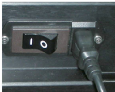
Figure 6-2 Main power switch and cable
