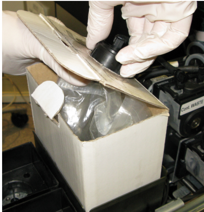
Figure 6-119 Attaching the waste drain tube
