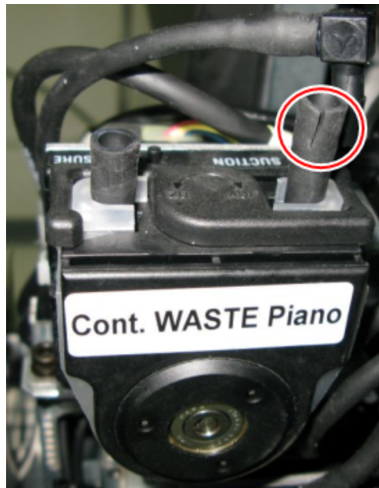
Figure 6-127 Tubes disconnected from the waste pump
