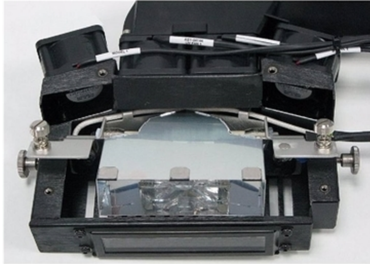
Figure 6-102 Removing the UV reflector from the UV assembly
