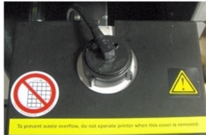
Figure 6-136 Cover installed on the waste container
