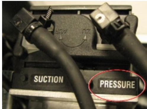
Figure 6-125 Tubes connected to the waste pump
