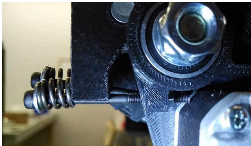
Figure 41: Tips of Bolts Bottomed Out on Motor
