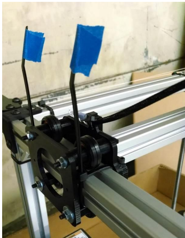
Figure 56: Cut the zip ties flagged with blue tape (qty 4)
