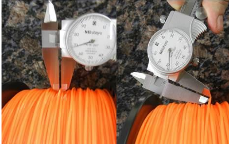
Figure 61: Measuring Filament Diameter
