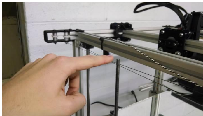
Figure 44: Checking XY Drive Cable Tension
