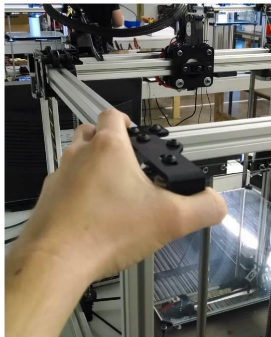
Figure 46: Re-aligning Idler Bracket
