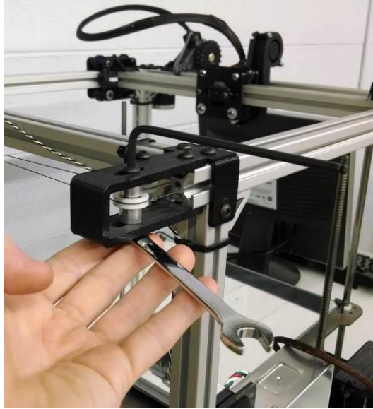
Figure 47: Adjusting the Idler Tension
