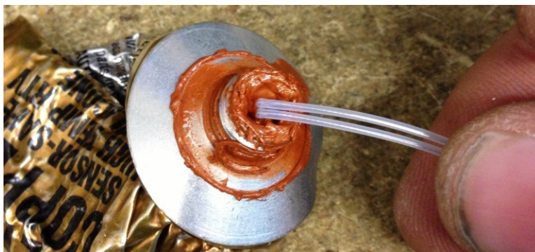
Fig. 3-8: Coating the thermistor with RTV.
