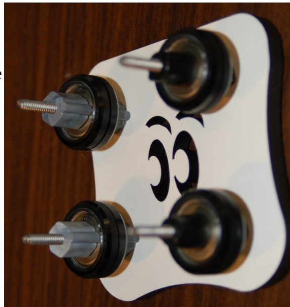
Fig. 8-21: Eccentric bearings installed.
