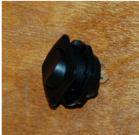
Fig. 16-46: The Power Switch.
