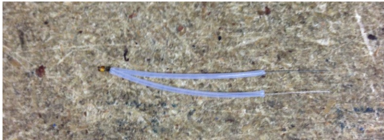
Fig. 3-6: Thermistor with PTFE sleeves installed.
