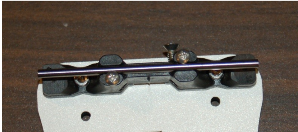
Fig. 8-15: Axle retaining screws installed.
