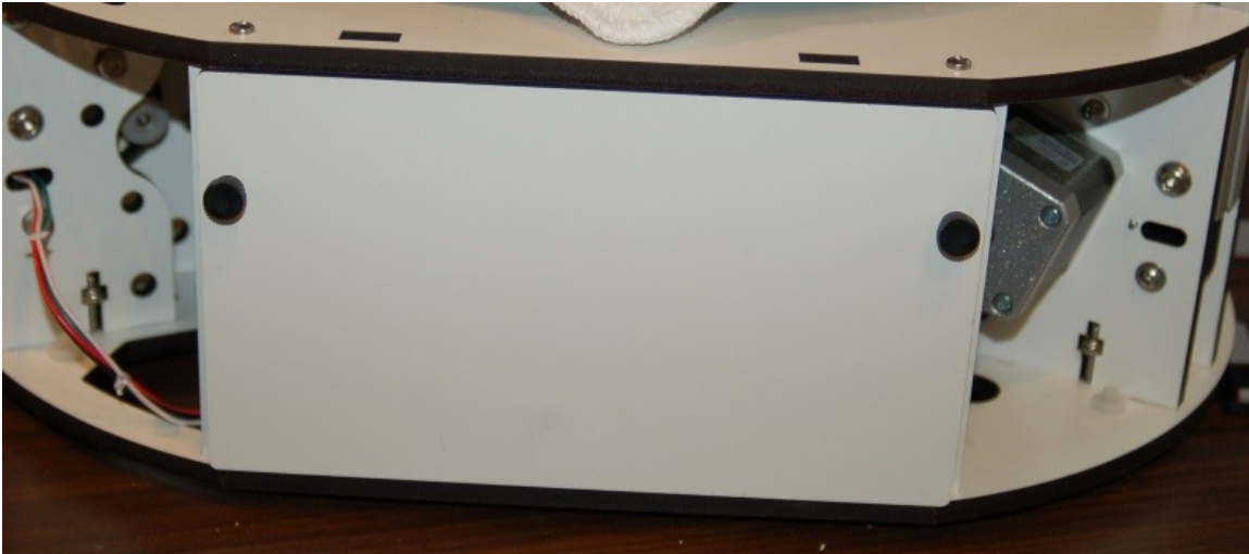
Fig. 17-1: Cover plate installed.
