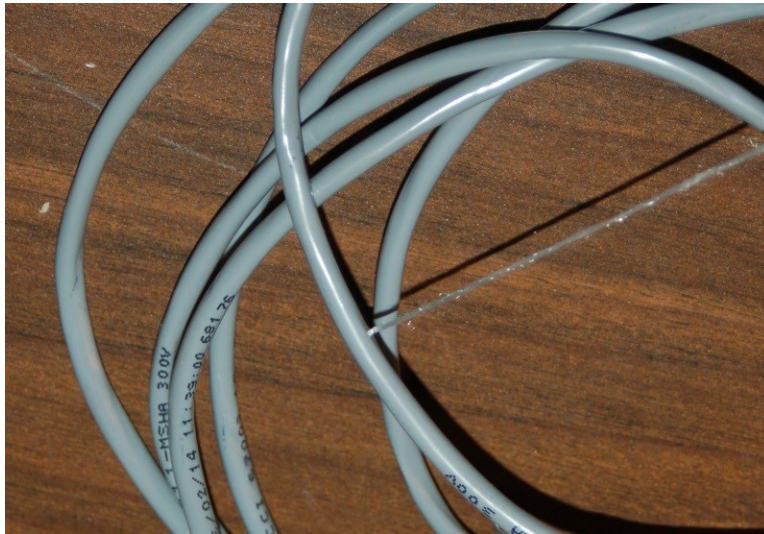
Fig. 6-1: Splitting the outer insulation.
