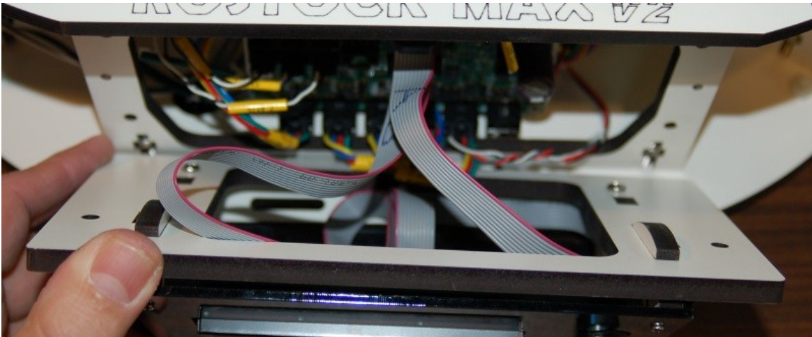
Fig. 17-3: LCD controller being installed.
