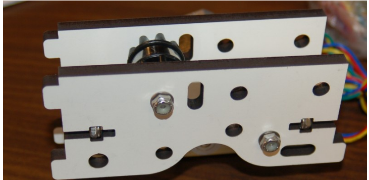
Fig. 4-40: Tower support installed.
