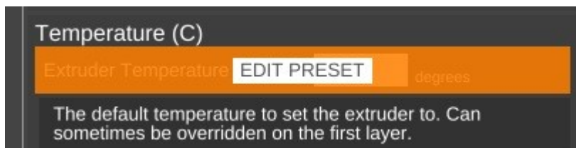
Fig. 22-16: Overriding a preset value.
