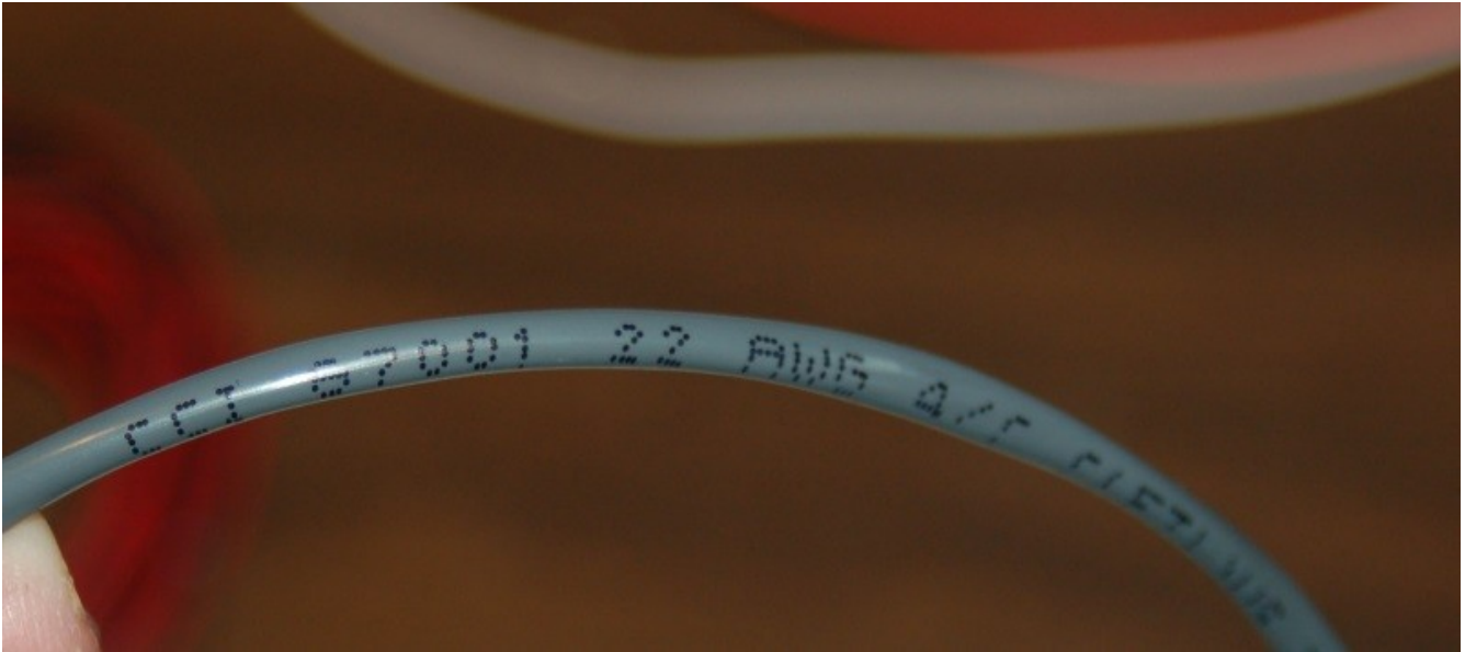
Fig. 6-10: Identifying the 22ga, 4 conductor wire.
