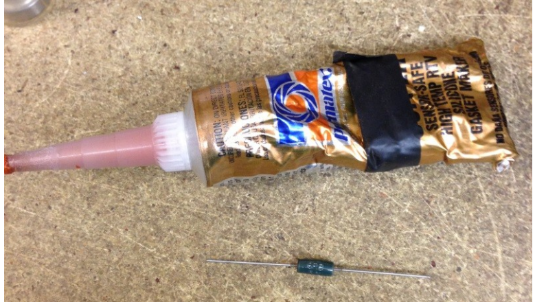
Fig. 3-2: RTV & heating resistor.
