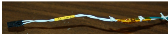
Thermistor leads finished & labeled.
