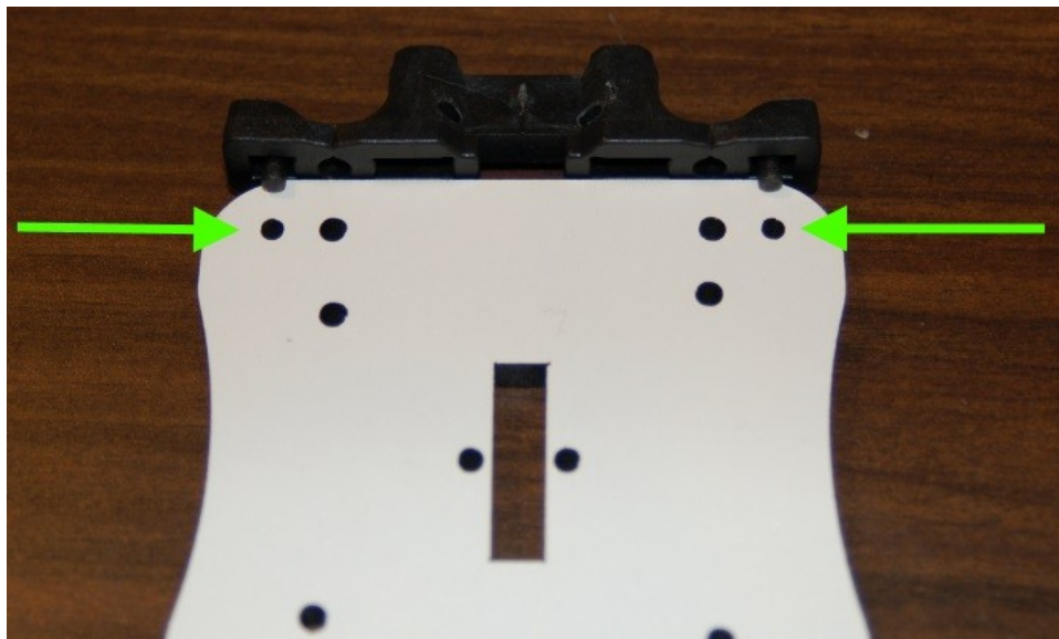
Fig. 8-6: U-Joint carriage installation location.
