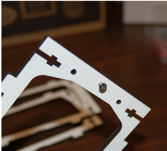
Fig. 4-6: Retaining screw installed.
