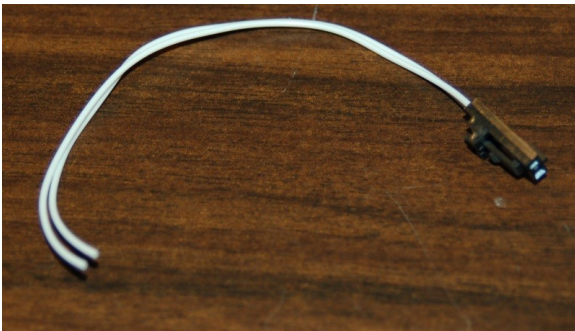
Fig. 16-19: Thermistor leads cut to length.
