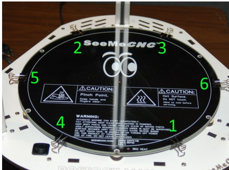
Fig. 17-20: Document clips installed.
