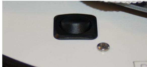
Fig. 16-49: Power switch installed.
