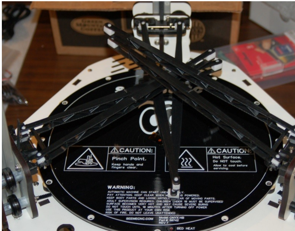
Fig. 12-15: All six arms installed.
