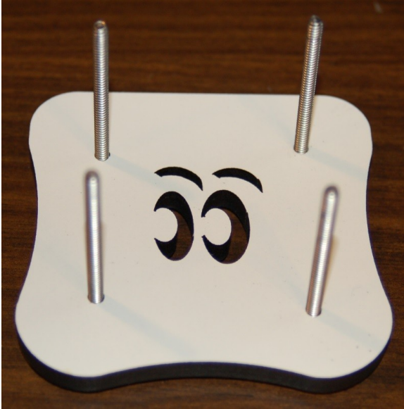
Fig. 8-19: Outer plate ready for bearings.
