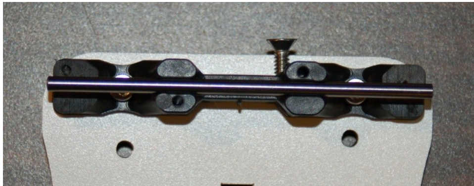
Fig. 8-13: Axle pressed into position.
