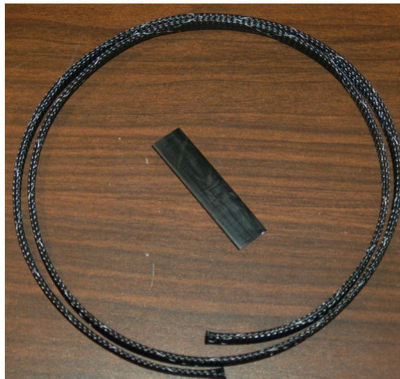
Mesh wiring loom and heat shrink tubing.
