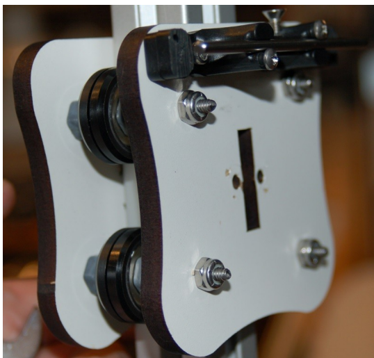
Fig. 8-24: Inner plate attached.
