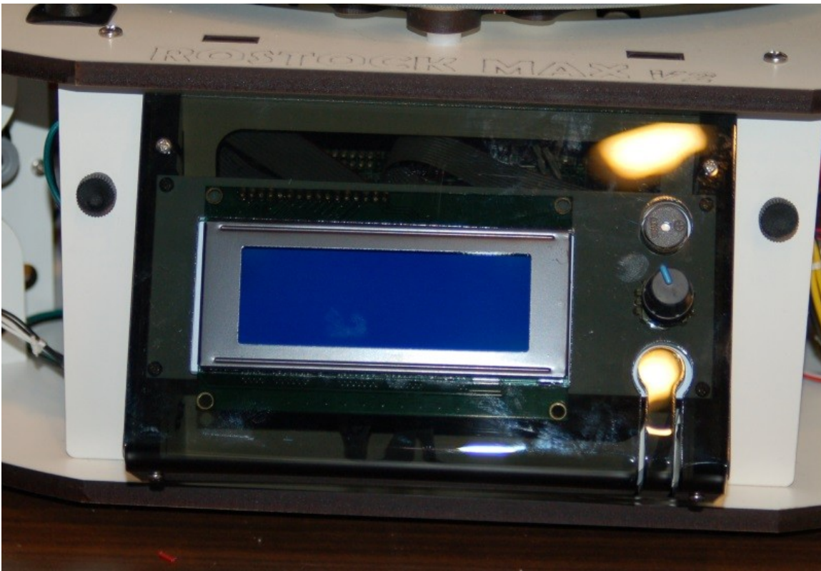
Fig: 17-4: LCD panel installed!
