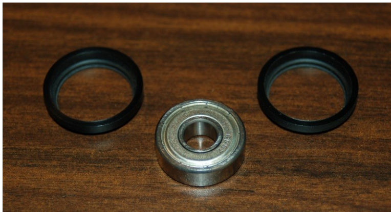
Fig. 8-1: 608ZZ bearing and two sleeve halves.
