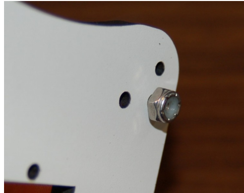
Fig. 8-9: Nylon lock nut installed.
