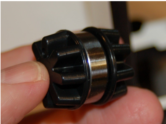
Fig. 7-19: Upper idler bearing.
