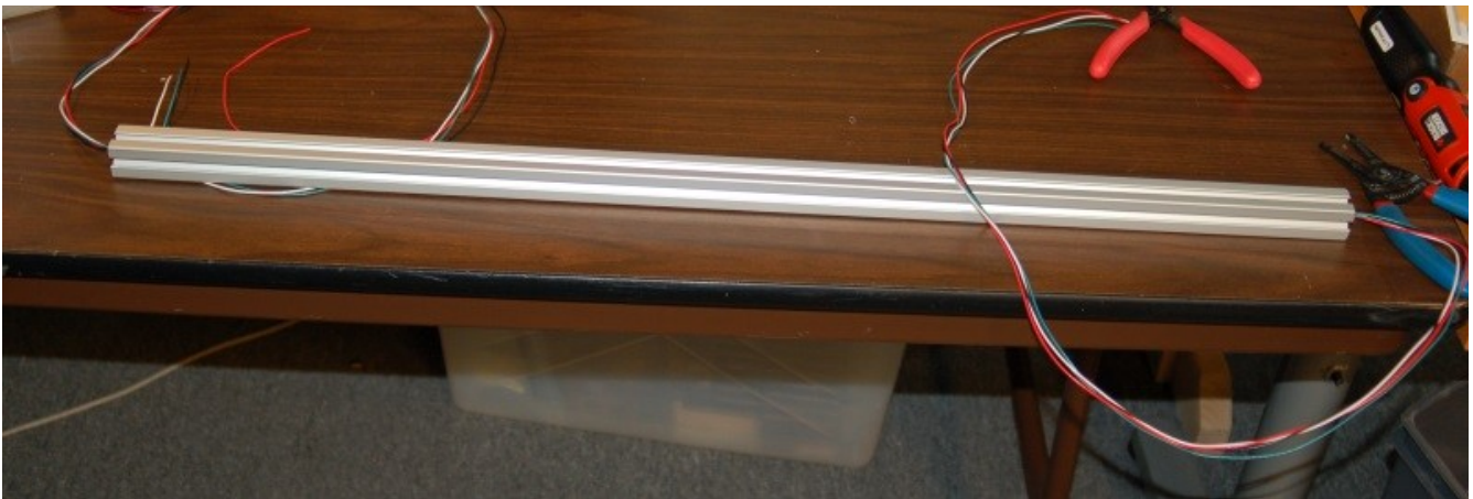
Fig. 6-3: 18ga wires routed.
