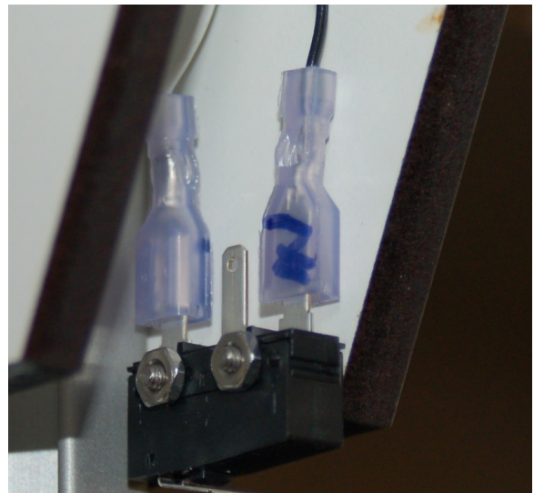
Fig. 7-34: Z axis end stop switch wired.
