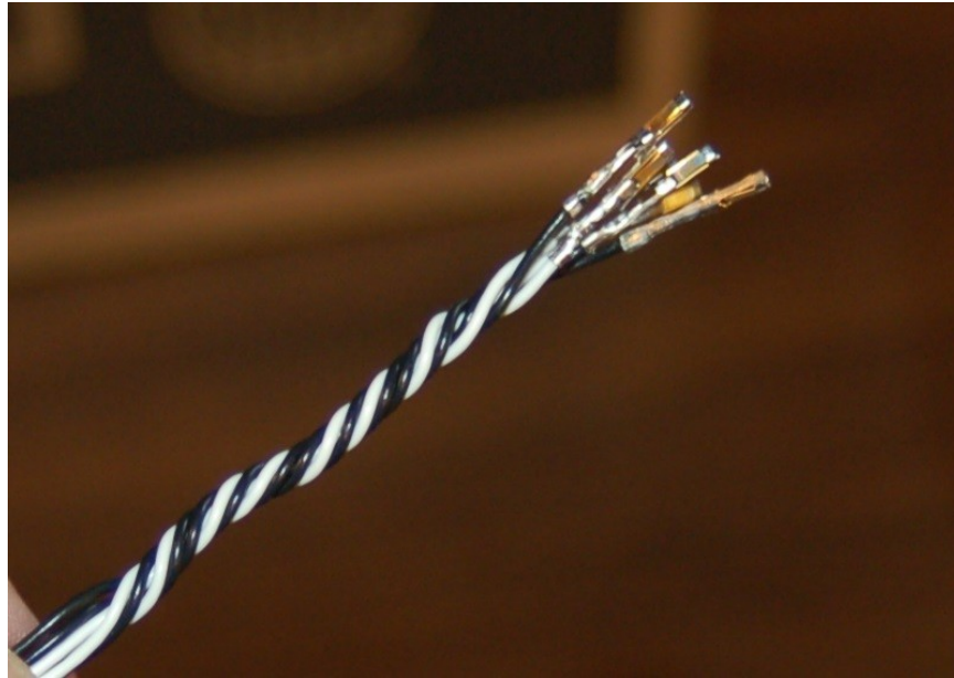
Fig. 6-4: End Stop wires bundled together.
