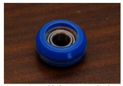
Fig. 9.1-3: Assembled carriage wheel.
