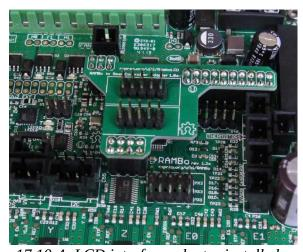
Fig. 17.10-4: LCD interface adapter installed.
