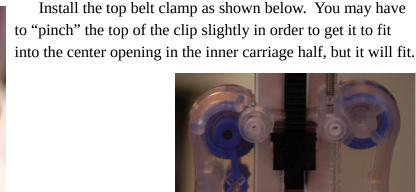
Fig. 9.6-2: Top clamp fitted.
