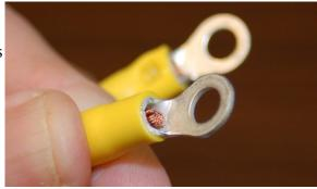
*Fig. 3.3-1: Proper wire position.*
