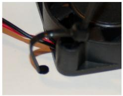
Fig. 17.1-2: Wire tie installed.
