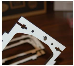
Fig. 6.2-1: Retaining screw installed.
