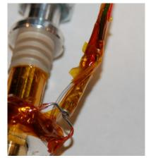
Fig. 11.3-12: Thermistor leads bound tight. (**Older wire style shown.**)
