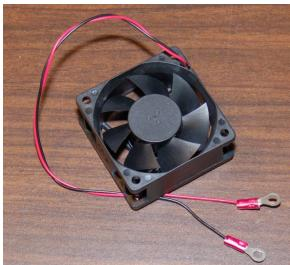
Fig. 3.3-3: Crimp connectors installed.
