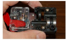
Fig. 10.1-7: Filament guide block orientation.
