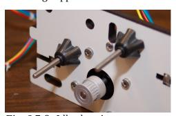
*Fig.* 6.7-8: *Idler bearing spacers*.
