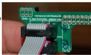
Fig. 17.10-3A: "A" & "B" cables installed (White PCB only!).
