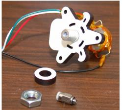
Fig. 11.4-1: Mounting plate in place.
