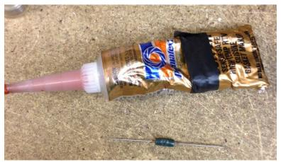
Fig. 3.1-2: RTV & heating resistor.
