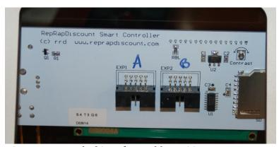
Fig. 16.2-4: Marked interface cable positions.
