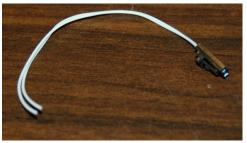
Fig. 17.4-1: Thermistor leads cut to length.
