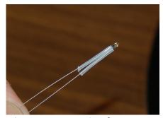
Fig. 4.1-2: PTFE insulators installed.
