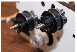
Now you can complete the assembly by fitting a tower support to the two screws. Install a #6-32 nylon lock nut to each screw – don't tighten it too much. Finger tight is fine. You want a bit of "wobble" in the assembly to assist in getting the top of the base installed.
