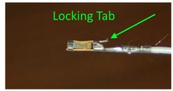
*Fig.* 17.3-1: *Female crimp connector.*
