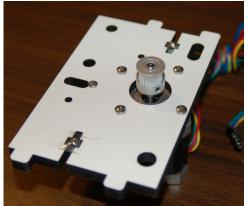
Fig. 6.7-4: First motor in place. Now install two #6-32 nylon lock nuts into the three tower supports as shown  $\overline{Fig. 6.7-5}$ : Motors installed!
