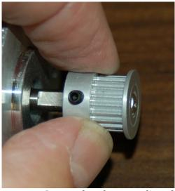
Fig. 5.1-2: Gear and grub screw aligned.
