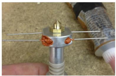
Fig. 3.1-4: Resistors installed in the hot end.
