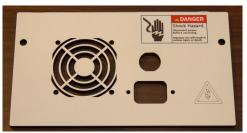
Install the IEC power connector using two 1", #6-32 pan head screws and two #6-32 nylon lock nuts.
