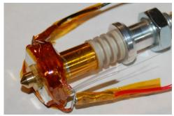
Fig. 11.3-10: Insulated crimps.
