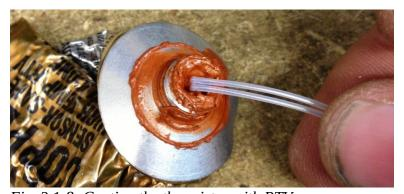
*Fig.* 3.1-8: *Coating the thermistor with RTV.*
