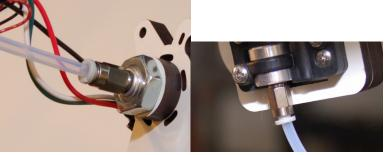
Fig. 11.5-3: Bowden tube fitted. ("**B**" wire shown."
