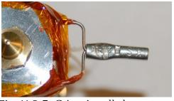
Fig. 11.3-7: Crimp installed.
