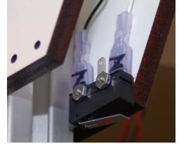
Fig. 8.7-3: Z axis end stop switch wired.
