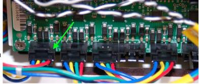
provided do not use this locking feature, *Fig. 17.8-6*: *Stepper motors plugged in.* so you need to make sure you insert the connector with the proper pin #1 orientation.
