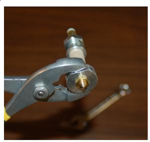
*Fig. 3.1-1: Tightening the nozzle.*
