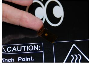
*Fig.* 4.1-1: Covering the thermistor hole.
