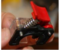
Fig. 10.1-2: Filament tensioner.
