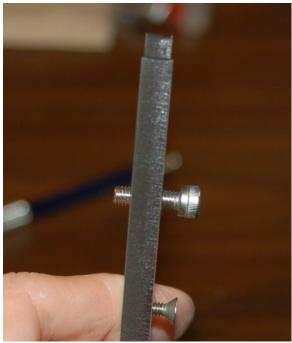
Fig. 6.2-6: "Tap" driven through completely.
