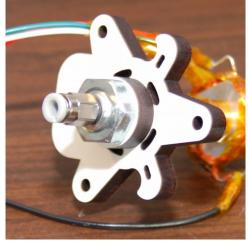
Fig. 11.4-2: Hot end tightened dwon.
