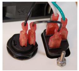
Fig. 6.6-7: IEC plug & switch wired.
