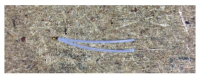
Fig. 3.1-6: Thermistor with PTFE sleeves installed.
