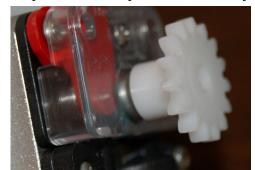
Fig. 10.2-7: Stepper knob installed.
