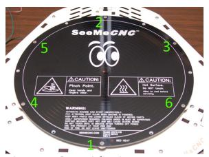
Fig 15.1-5: Screw tightening pattern.
