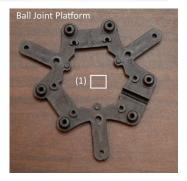
Do NOT sand or de-burr the ball joint arms or the sockets in the delta arms! Doing so will ruin the fit of the parts!
