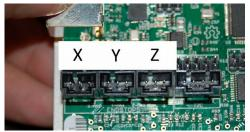
Fig. 17.8-1: End stop connector plugs.
