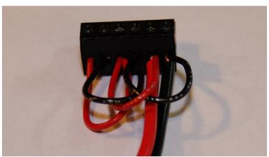
Fig. 3.2-3: RAMBo power connector completed.
