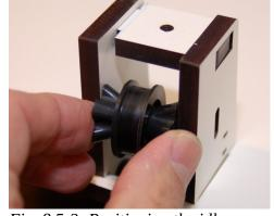
Fig. 8.5-2: Positioning the idler assembly.
