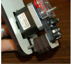
Fig. 10.2-5: Fitting the EZStruder to the bracket.
