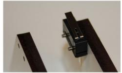
Finally, install one #2-56 finish nut on to each mounting screw. Use a little bit of thread-locker here.
