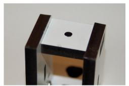
Fig. 8.2-7: Spreader fully seated.
